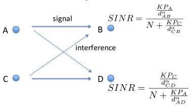
$P_A$  etc are transmit powers.  $d_{AB}$  are distances. Log-distance path loss model is used. There is a link between AB or CD if the corresponding SINR  $\geq \beta$ .
