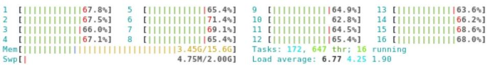
Computational complexity of H.264 decoding a 8K video in a Chrome browser on an Intel i9–9900K CPU with 3.60GHz and 16 cores. Even with 800% CPU usage, Chrome was not able to render the video.
