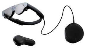
Magic Leap 2HoloLens 2Resolution1440 x 1760 per eye1440 x 936 per eyeOpticsWaveguideWaveguideRefresh Rate 120 Hz60 HzField of View 70° diagonal52° diagonal
