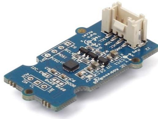
Accelerometer, Gyroscope, Magnetometer
